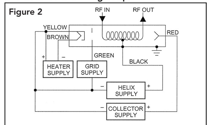
The Ring Loop TWTs are best known for an ability to amplify microwave signals simultaneously over a radar band of frequencies. A Ring Loop TWT is illustrated schematically in Figure 2, which also shows the power supplies to operate the TWT. This TWT consists of an electron gun (composed of a heater, cathode, and control anode), a helix (slow-wave structure), an attenuator, a collector, and an input and an output coupling element
