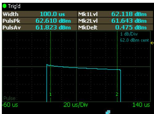
Figure 15 Power at 100  $\mu$ s pulse width and 1 kHz pulse repetition frequency
